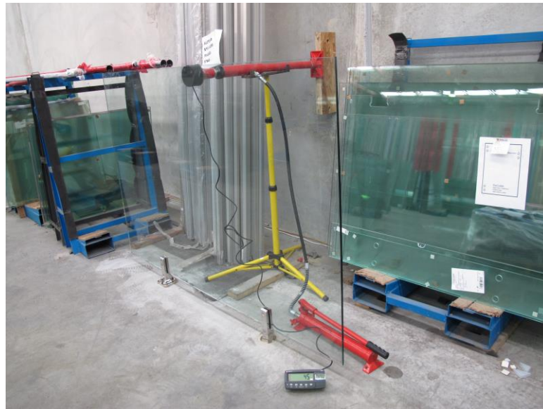
Square Core Drilled spigots under the test.
